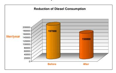
250 KVA, 8 years old generator were sold for 4000 USD and exchanged for a 500 KVA at 42000 USD new generator as a CP options at Sevenplast which is illustrated below:
